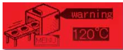
Warning screen during material shortage, etc.
